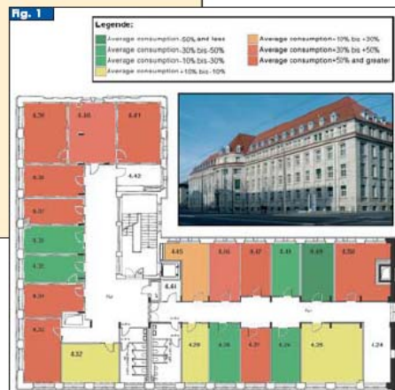
The LAS GmbH office block in Leipzig with the 'energy traffic light' - room-by-room consumption ranking
